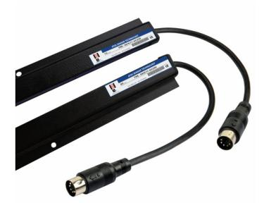
ATEK 987 series door security detectors can read from 4 meters distance. With 36 built-in photodiodes with fast response speed, they provide fast security. There is external power unit working with 220VAC power supply.
